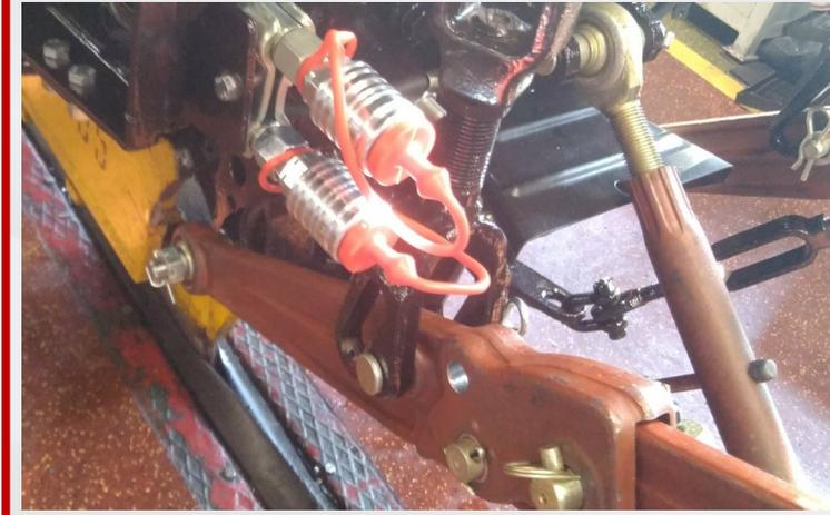
MQS-AF ISO A Push-Pull Female -08 installed closed view. MQS-A ISO A Males -08 are also used.
